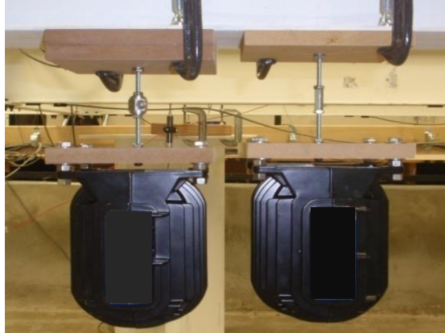
Figure 6.13. Suspended force transducer and TT with stinger type setup (left) and arrangement without force transducer (right). (Photo by EVF, dynamics lab, 7/9/13)
