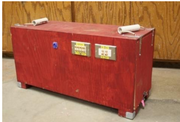
Figure 7.8. Photograph of field ruggedized amplifier enclosure. (Photo by EVF, dynamics lab, 10/18/13)
