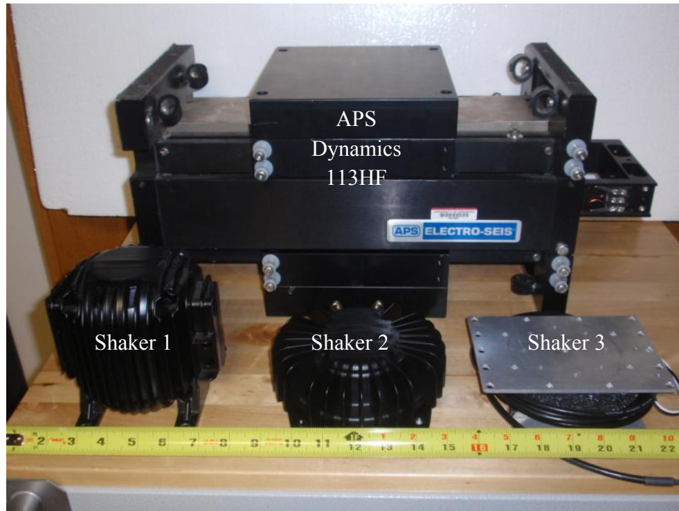
Figure 2.1. Shakers evaluated for use in MIMO EMA. (Photo by EVF, dynamics lab, 9/14/12)
